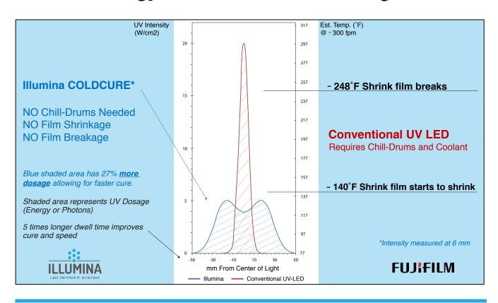
As illustrated in the chart above, the UV dosage of the Illumina COLDCURE process is below the 140°F indicator line where shrink film begins to shrink, so heat and its effects are taken out of the equation. The COLDCURE benefits of Ultra Low Temperature plus High Dosage and Dwell Time are numerous.
